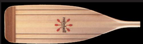
The **Mitchell Saco Paddle** is a touring canoe paddle for open boat paddling on lakes, rivers and streams. This is an economy paddle with the solid construction for which the Mitchell name is known. The shaft is solid spruce and the blade is laminated basswood, maple, and beach. The blades are 7" wide and 20" long and protected with an internal hardwood tip covered with a veneer. The handle is a palm grip and an integral part of the shaft. The stock sizes are 54", 57", 60", and 63".
